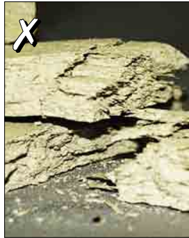
Broken asbestos insulating board, asbestos lagging and sprayed asbestos (limpet)
